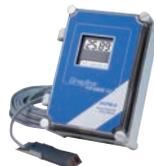
**Ultrasonic Open Channel Flowmeters** typically measure the depth of water flowing through a flume or over a weir. The sensor is mounted above the water surface and bounces a signal off of the surface to measure the relative depth. The water depth correlates to a specific flow rate for the specific flume or weir configuration.
