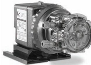
This squeezing action of the flexible tubing generates a powerful vacuum that moves both gases and liquids simultaneously, without the pump losing its prime. The pumps are completely self-priming up to 25 feet, can operate dry and will not clog from dirt and minor debris.
