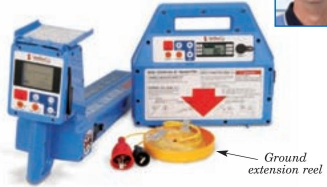
Connect the ground extension lead end to a valve, hydrant, or other connection farther down the pipe you want to locate. Make sure that the wire from the ground extension reel is placed at least 10 feet away from the pipe you are locating so you don't pick up any interference.
