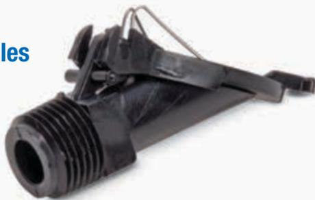
This economical non-clog foam control spray nozzle produces a wide bank spray pattern while using minimum pressure and water volume. Only 2.7 psi of pressure and 2 gpm flow provides a wide, flat spray pattern 60" wide at a distance of 18" from the nozzle tip. This nozzle can handle contaminated liquids as the cap is spring loaded. Should the nozzle become clogged, just lift the cap to purge any blockage.
