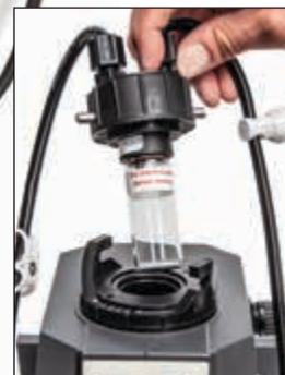
Ultrasonic autoclean system keeps the optical glass cuvette chamber clean.
