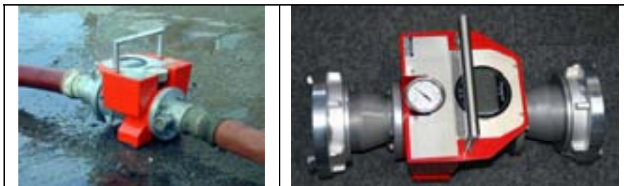
Picture 7: Inline use of Flowmaster and a Flowmaster with fittings for use with Hoselayers. Photos courtesy of Essex County Fire and Rescue Service and Greater Manchester Fire and Rescue Service respectively
